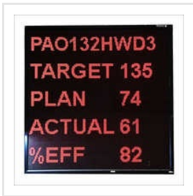
Production Monitoring Display System
